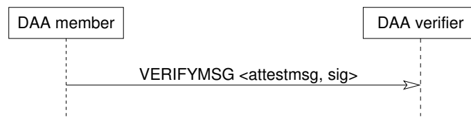
Figure 4.4: Protocol to send an attestation message to the verifier
